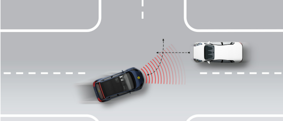
Test car turns across the path of an approaching car
